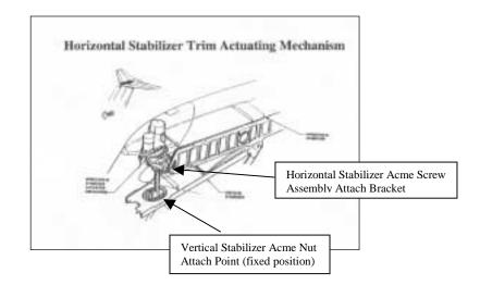
The MD-80 and DC-9 derivative aircraft utilize a single Acme screw / nut assembly to provide longitudinal trim control. This design incorporates an internal titanium torque tube as the Acme screw drive mechanism and redundant load path. The DC-8 aircraft, however, utilizes a dual Acme screw / nut assembly such as described above. Redundancy is provided through the dual assemblies. No torque tubes are used in the DC-8 design.
