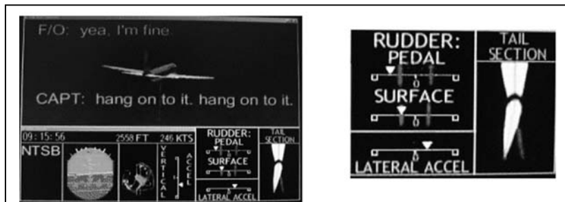
The rudder reversal before the “bang” sound on the cockpit voice recorder and the tailfin separated. Rudder pedal position is shown exceeding the movement limits, but the rudder travel is not. A later frame showing the rudder in a slightly out-of-bounds position may be an artifact resulting from the use of filtered data. The unfiltered DFDR trace of rudder position does not show it moving out of limits. Source: NTSB
