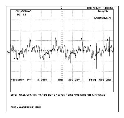
It's interesting to note that the Ground plane Interference EMI Specification for the FA-18 is < 1 volt RMS above 500 Hz. This is to avoid damage to the Avionics, I learned in a phone call to a Boeing expert.
