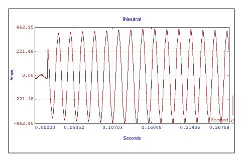
Interestingly, during faults in which a phase opens and causes current to flow over structure, the structural current path mirrors the routing of the power conductors. This is known to cause arcing at conduit joints. This is one of the reasons why the NEC considers an AC distribution system with a multiple grounded neutral to be a fire hazard.
